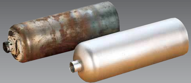
Cylinder surface profiled with aluminum oxide
