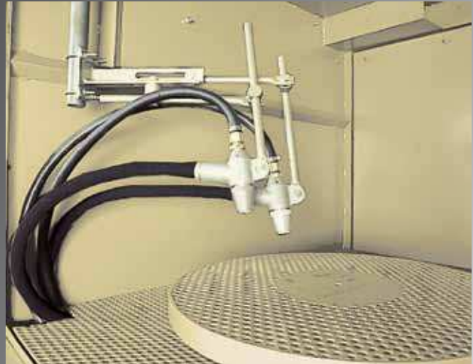
Fixed gun holder frees operator to manipulate parts.
